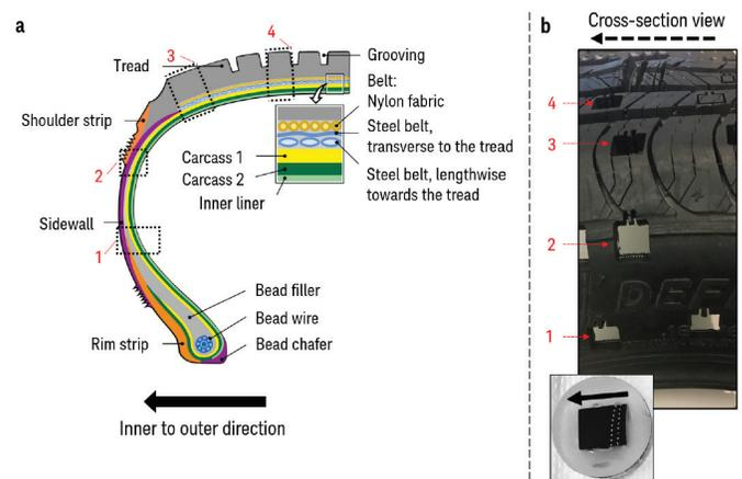
**Figure 1. (a) Schematic of cross-sectional view of the tire structure containing layers of different materials. Locations are marked as 1-4 from different regions of tire. (b) Samples cut from locations 1-4 (top) and a mounted and polished sample in epoxy for nanoindentation test (bottom) with an arrow showing the direction of indents performed on the cross section of the tire.**
