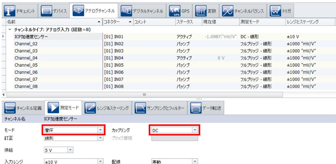
The screenshot displays the software interface for configuring an ICP acceleration sensor. The top menu bar includes options like 'Analog Channels', 'Digital Channels', 'GPS', 'Variables', 'Channel Balance', and 'Triggers'. The main window shows a list of channels under 'Analog Input (Total=8)'. Channel 02 is selected, and the 'Measurement Mode' tab is active. The configuration for Channel 02 is as follows:
