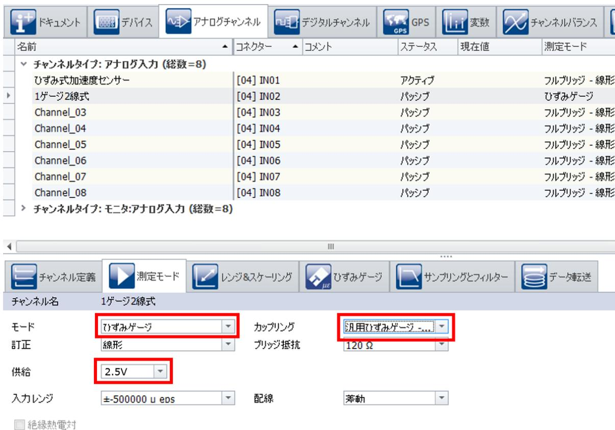
The screenshot shows the software interface for configuring measurement channels. The top part displays a list of channels under 'チャンネルタイプ: アナログ入力 (総数=8)'. The bottom part shows the '測定モード' (Measurement Mode) configuration for a selected channel '1ゲージ2線式'. The settings are as follows:
