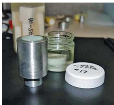
Figure 2. Phantom tissue as mounted for testing in fluid.
