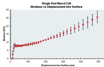
Figure 5. Modulus for the four indents in a single RBC.
