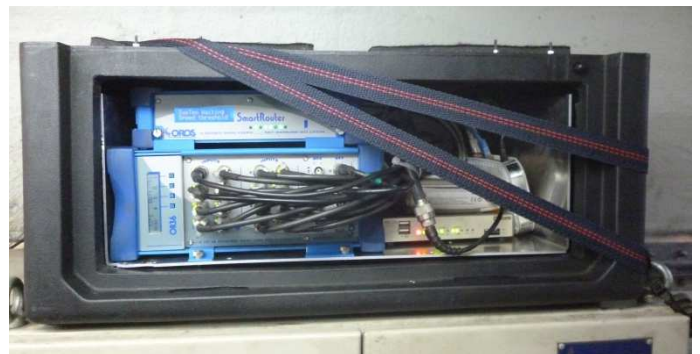
Fig. 4: Satellite system with 3G and WIFI modems in the DOCK PACK package
