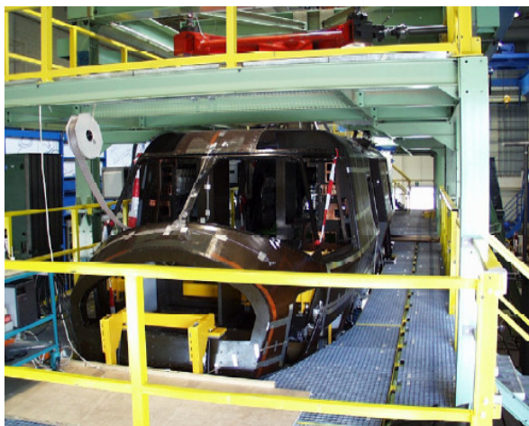
Tests mainly involve strain gauges and displacement signals
