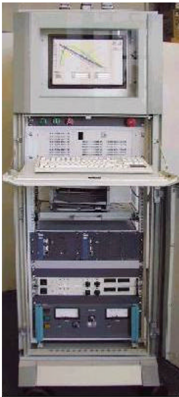
Test rig control unit with measurement system and motor power excitation
