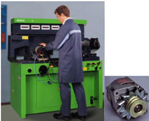
A BOSCH car dynamo test stand and a tested dynamo
