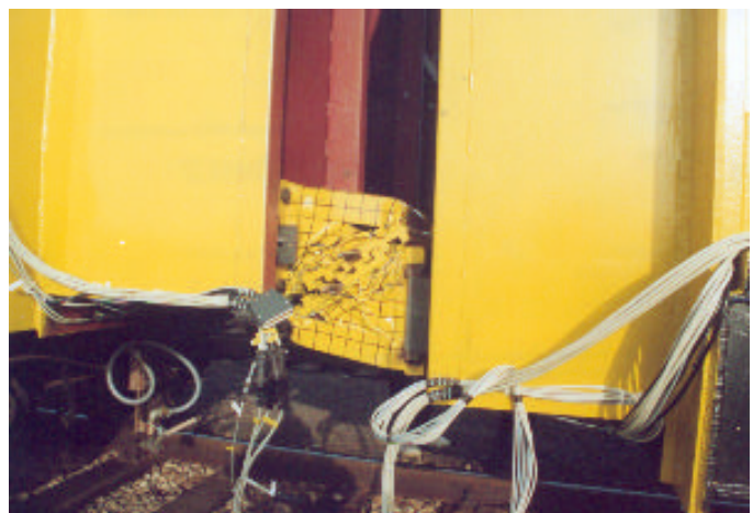
After the crash the buffers are destroyed
